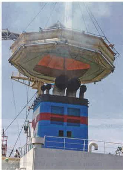
A 2,500-pound bonnet caps a chemical cargo ship's smokestack and collects toxic pollutants, which are delivered by flexible ducts to a treatment system at the Port of Long Beach.
